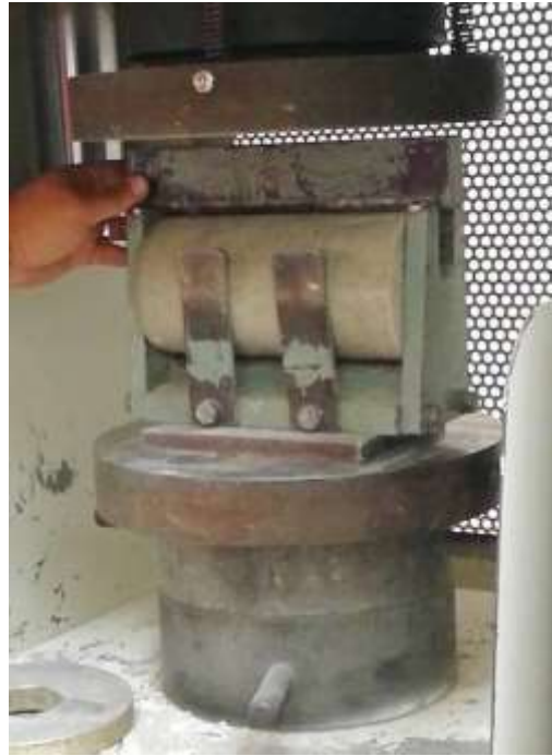
Figure 3. Splitting tensile test arrangement
