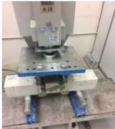
Figure 1. Flexural test of LFC
