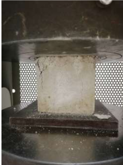
Figure 2. Compression test of LFC
