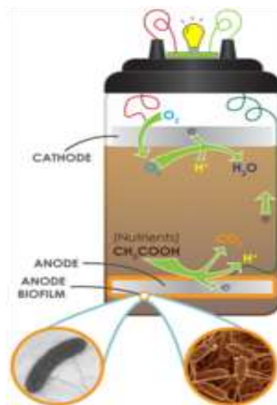
Fig. 3 A model of a Soil-Microbial Fuel Cell (Source: Wikipedia, 2011)
